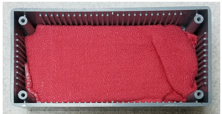
View showing the inside of the Box, will cloth to support the Batteries
